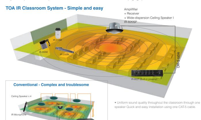
Assembled specifically for classroom use, TOA's new Infrared Wireless Classroom System includes a ceiling-mounted widedispersion speaker (with integrated receiver and amplifier), an easily accessed desktop tuner and a pair of lightweight IR wireless microphones, one each for the teacher and students.
